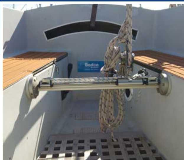
Barton's removable mainsheet system creates more space in the cockpit
