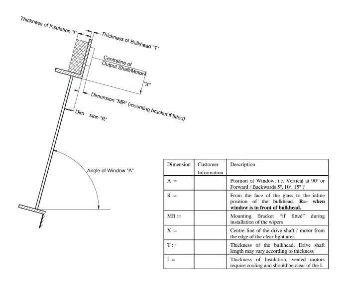
Dimensions; A, R & MB are required for us to select the correct spring pressure in the wiper arm. We will manufacture our product with the correct blade pressure on the glass to give an efficient window wipe.
