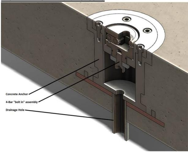
Top fixing Helicopter Tie-Down with stainless steel housing c/w drain.
