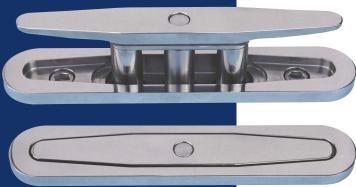
A range of manual and power operated Flush Fitting Automatic Retractable Cleats has been developed. The cleat has two positions, stowed and raised ready for use. In the stowed position the entire cleat and base is flush with the deck.
