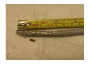
2. Carefully peel back the braid and trim back to insulation.
